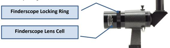
Once focused, then align your finderscope by gently adjusting the two thumbscrews on the finderscope bracket (the silver "knob" contains a spring that gives backpressure to the thumbscrews and does not need adjustment). Carefully align the finderscope body until its crosshairs are centered on the object that is currently centered in the main telescope's eyepiece.
