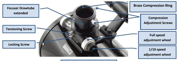
The Apertura focuser will accept 2" and 1.25" eyepieces (with included adapter) and other common hardware. The amount of extension required for each eyepiece will vary,
